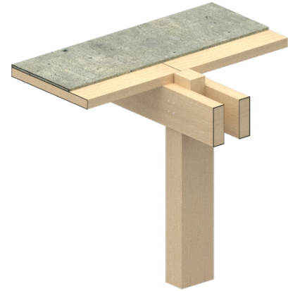
Figure 1.01 Mass Timber System Isometric (Library Load Areas)
